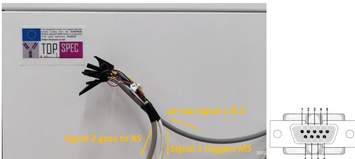
**Figure 2.** Leads connection among autosampler, pI trap and MS. Two of the 9 leads from the pI trap that transmit signal 1 and ground are connected to MS triggering cable. All the leads except for signal 1 are connected to the autosampler corresponding leads.
