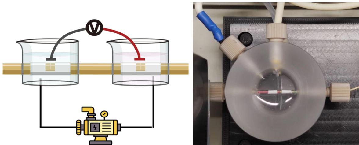
**Figure 1.** Upgraded pI cell. Nafion membrane and PEEK tube are connected by heat-shrink tubing. Electrode and tubes from and to the peristaltic pump are attached to the cell.
