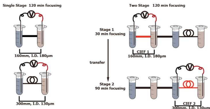
**Figure 6.** Design of a one- and two-stage pI cell, respectively. For the two-stage cell, it is critical to assure both cells have the same volume. Potential is applied to the two cells sequentially.
