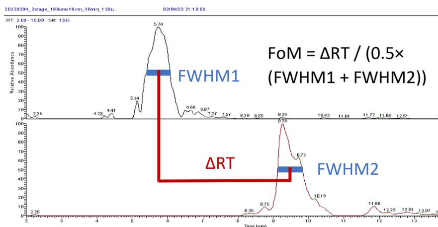
**Figure 5.** Formula for calculating FoM. The full width at half maximum (FWHM) is measured separately for two peaks. FoM is calculated letting the difference in retention time to be divided by the average of two FWHM. The larger the FoM is, the better the two proteins are separated.
