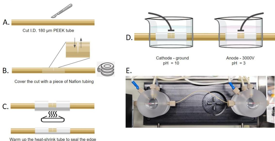
**Figure 9.** Assembly of a new machine pI cell. A-C: step-by-step procedure of preparing one side of the tube. D-E: let the tube partially go through the machine cell followed by installing the electrode and peristaltic tubings to accomplish the assembly.
