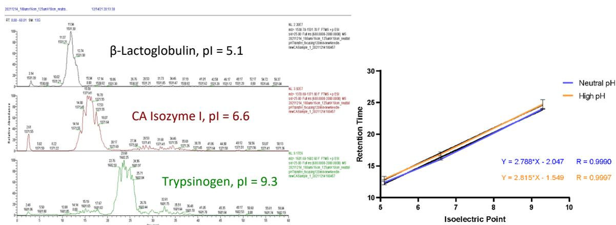
**Figure 4.** Left: The retention time and intensity of three proteins after 30-minute isoelectric focusing. No evident dispersion or asymmetric peaks was observed. Right: The linear correlation of proteins' retention time vs isoelectric points, among 3 replicates. R values are both  $\geq 0.999$  with neutral or basic transfer buffer pushing the sample.
