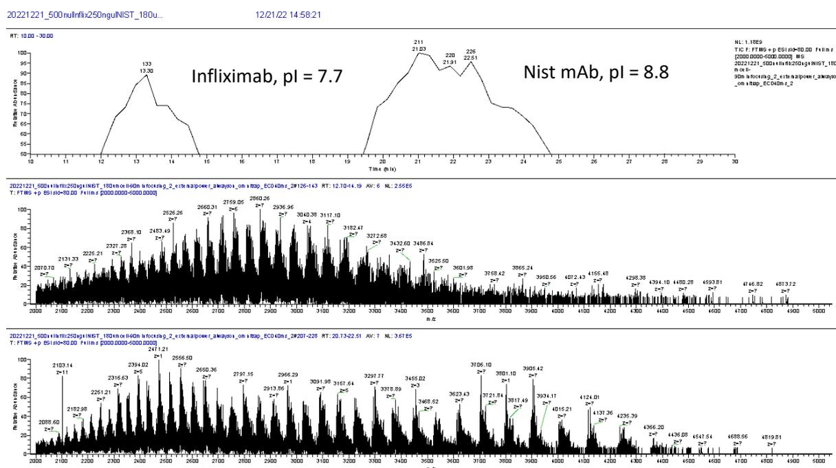
**Figure 8.** The separation of infliximab and NIST mAb after 90-min cIEF in pI cell, and their full MS spectrum.
