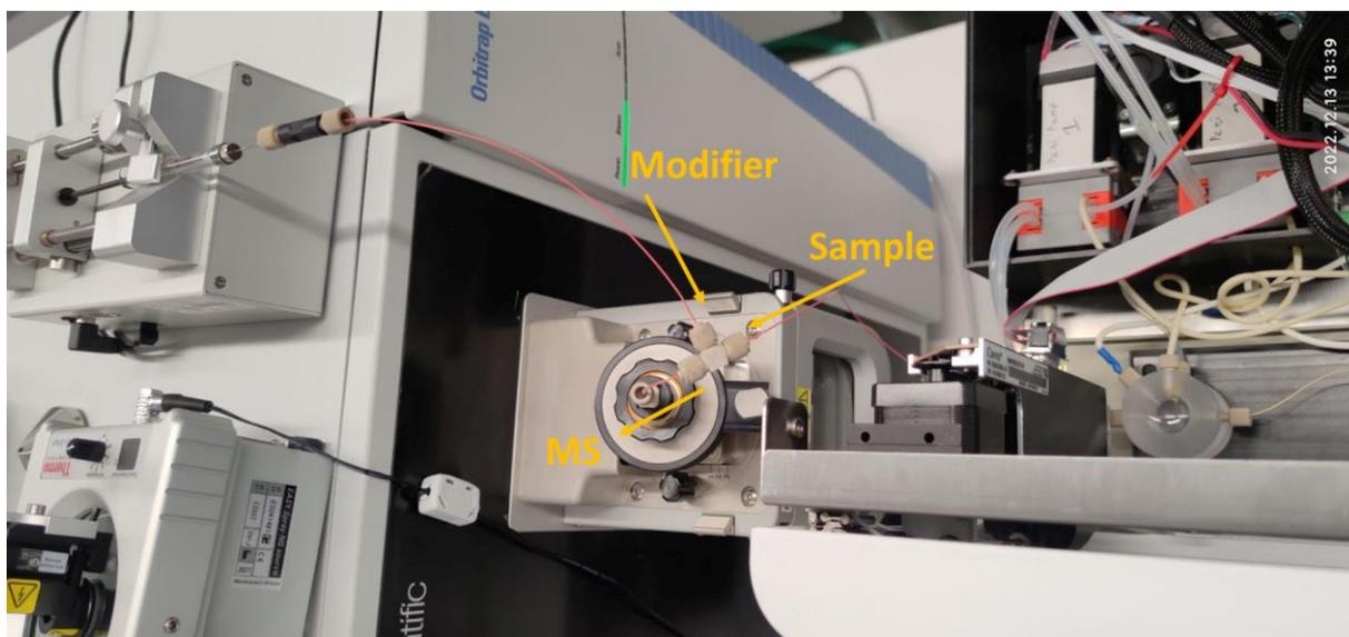
**Figure 3.** The introduction of modifier to the sample after cIEF. A tee connector is employed to facilitate the mixing.
