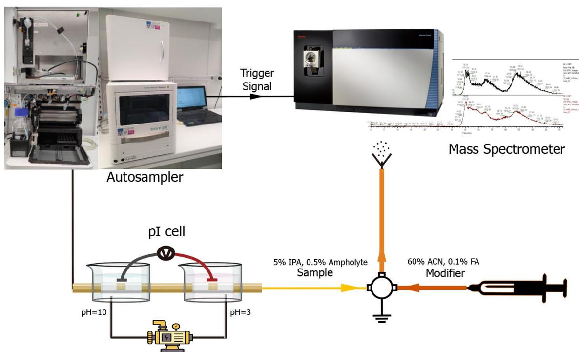
**Figure 10.** The current setting of tested, optimized pI-Trap-ESI interfaced with MS.
