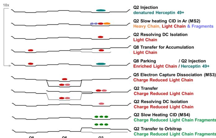
**Figure 3:** Ion processing steps in an MS4 top-down workflow for the analysis of intact mAbs involving slow-Heating CID of charge reduced ECD precursor ions.
