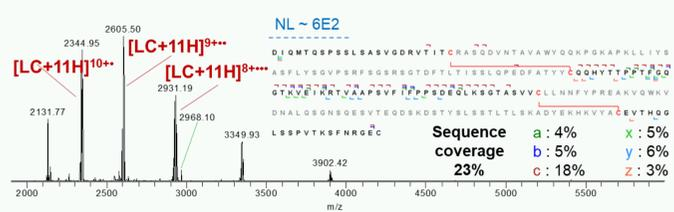
**Figure 8:** MS3 ECD mass spectrum showing charge-reduced LC ions serving as the precursor species in the MS4 step. Also shown is the sequence coverage obtained by extending ECD reaction time to enhance dissociation of the LC.
