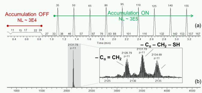
**Figure 7:** (a) TIC plot showing enrichment of the LC ion population in accumulation mode and (b) the isolation window highlighting variations on the cysteine side chain generated upon intermolecular disulfide bond cleavage by CID.
