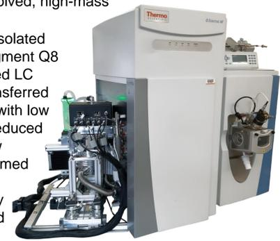
**Figure 4:** The Omnitrap platform coupled to a Q Exactive Orbitrap Mass Spectrometer.
