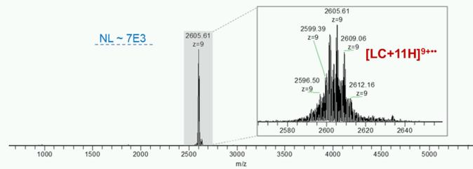
**Figure 9:** Mass spectrum showing the isolated charge-reduced LC ions formed by electron capture at MS3 level.
