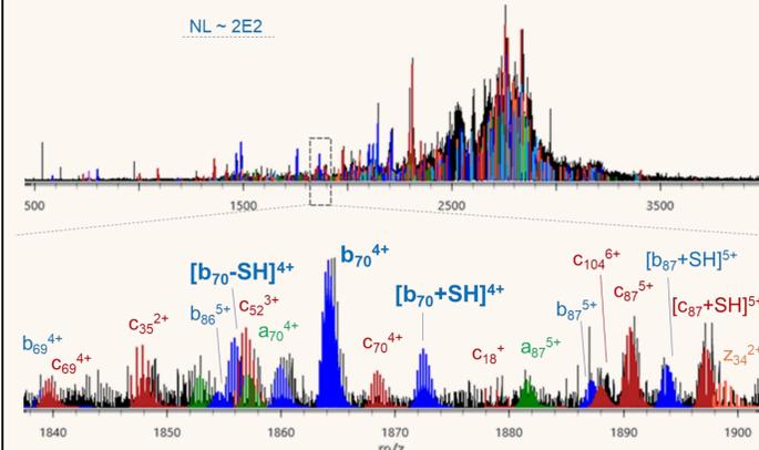
**Figure 10:** Annotated MS4 CID mass spectrum highlighting the triplet fragment ion configuration arising from the dissociation of the first intramolecular SS bond.
