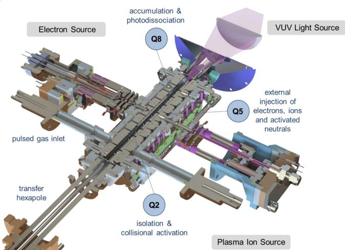
**Figure 2:** The Omnitrap platform is a segmented RF linear ion trap enabling multidimensional multiple-stage tandem mass spectrometry.
